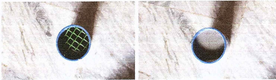
Fig. 5. Improvised sediment trap used to catch sediments installed near the soft bottom.
